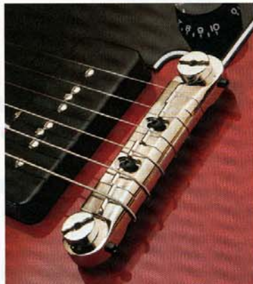
Wilkinson's latest wrapover bridge has two lockable sliding centre sections for fine-setting the intonation
